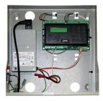
Pre-wired with 3 Amp PSU in metal case with tamper switch and circuit
