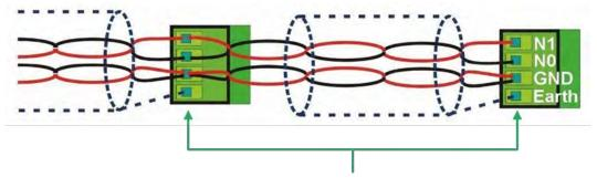
The screen for each cable must only be connected to the electrical earth at one end, otherwise ground loop currents may be introduced
