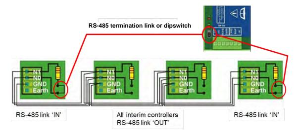
It is possible to connect using a star arrangement provided that RS-485 hubs are employed.
