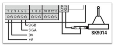
The SK9014 antenna is an optional item that may be required when the transmit distance surpasses 4m (line of sight).
